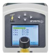
Other important color scales, including **Hunter L,a,b** and **CIE L\*a\*b\*** are provided within the firmware, allowing for the capability to use your ColorFlex® EZ Citrus to measure the reflected color of a wide range of non-citrus samples - liquids, semi-solids, powders, and solids.
