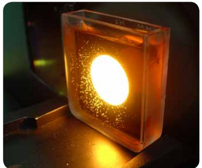
Figure 3. 10 mm Transmission Cell with typical liquid sample measured for Gardner Index.
