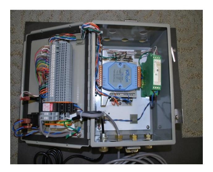
The end user will connect the wiring (two wires for each channel) at the terminal strip on the inside door of the support unit. There are 4 channels: 3 for color, and 1 for an index such as DE. The color channels are numbered 1-3 and will always be in the same order as the display. For example L a b, X Y Z, etc. are channels 1 2 3.
