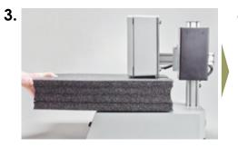
Place center foam with lid on top of workstation. Push center foam to back of the sensor until the notch in foam firmly engages with vertical support. Lower sensor tight against center foam lid. Retighten the adjustment handles.
