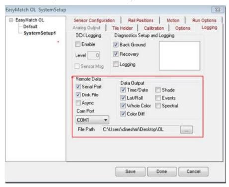
**STEP-3:** Remote Data output sends data to a COM port or a file, only if *Write to Lot File* option is checked in *Run->Product Setup->EasyMatch OL Productsetup->Page3*.
