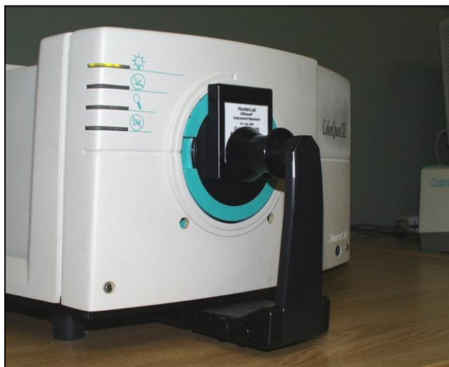
Figure 14. Setting Top of Scale with the White Tile
