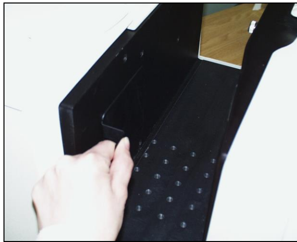
Figure 13. Setting Bottom of Scale for RTRAN Mode
