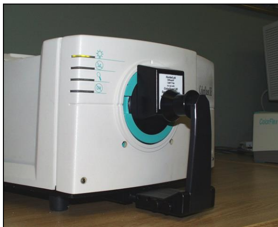
Figure 11. Standardizing on the Light Trap to set Bottom of Scale
