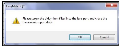
Figure 211. Didymium Filter Test: Place filter at RTRAN port
