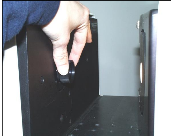
Figure 212. Inserting the Didymium Filter at RTRAN port (lens side)
