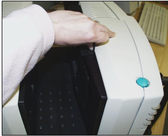
Figure 12. Setting Bottom of Scale for TTRAN
