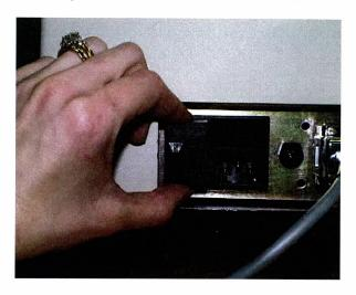
3. Pull back the tab to release the fuse holder.
