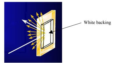
Light interactions for a transparent sample measured in reflectance
