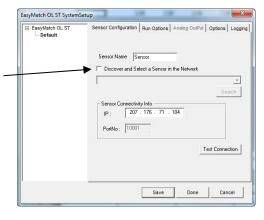
C. When the sensor serial number has been found and the IP address matches, then press 'Save' and 'Done'. The message, '*Please select a System Setup to Edit*' should then stop blinking.
