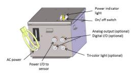
E. If an analog output device is to be used, connect the analog output end of the analog output-support unit cable to the output device.
