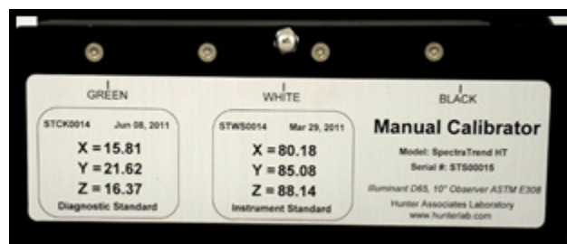
Figure 1-2. Calibrated Values for the Slide-On Calibrator
