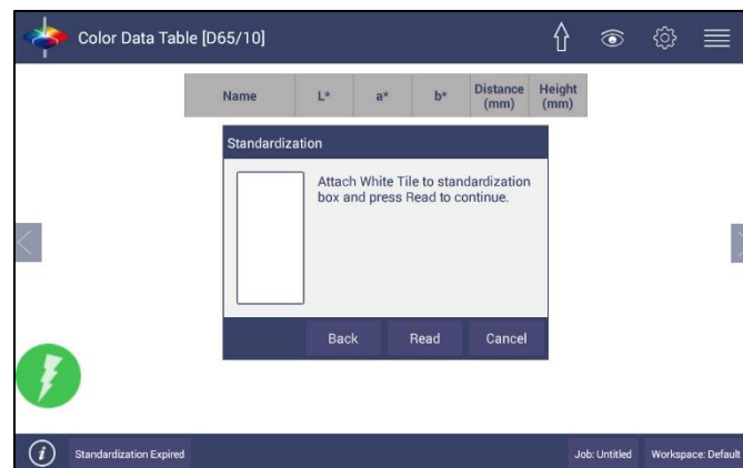
Figure 7. Read the White Tile for Top-of-Scale
