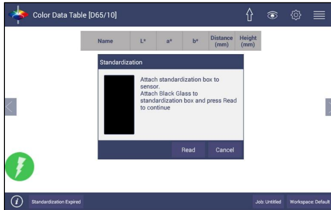
Figure 6. Read the Black Glass for Bottom-of-Scale
