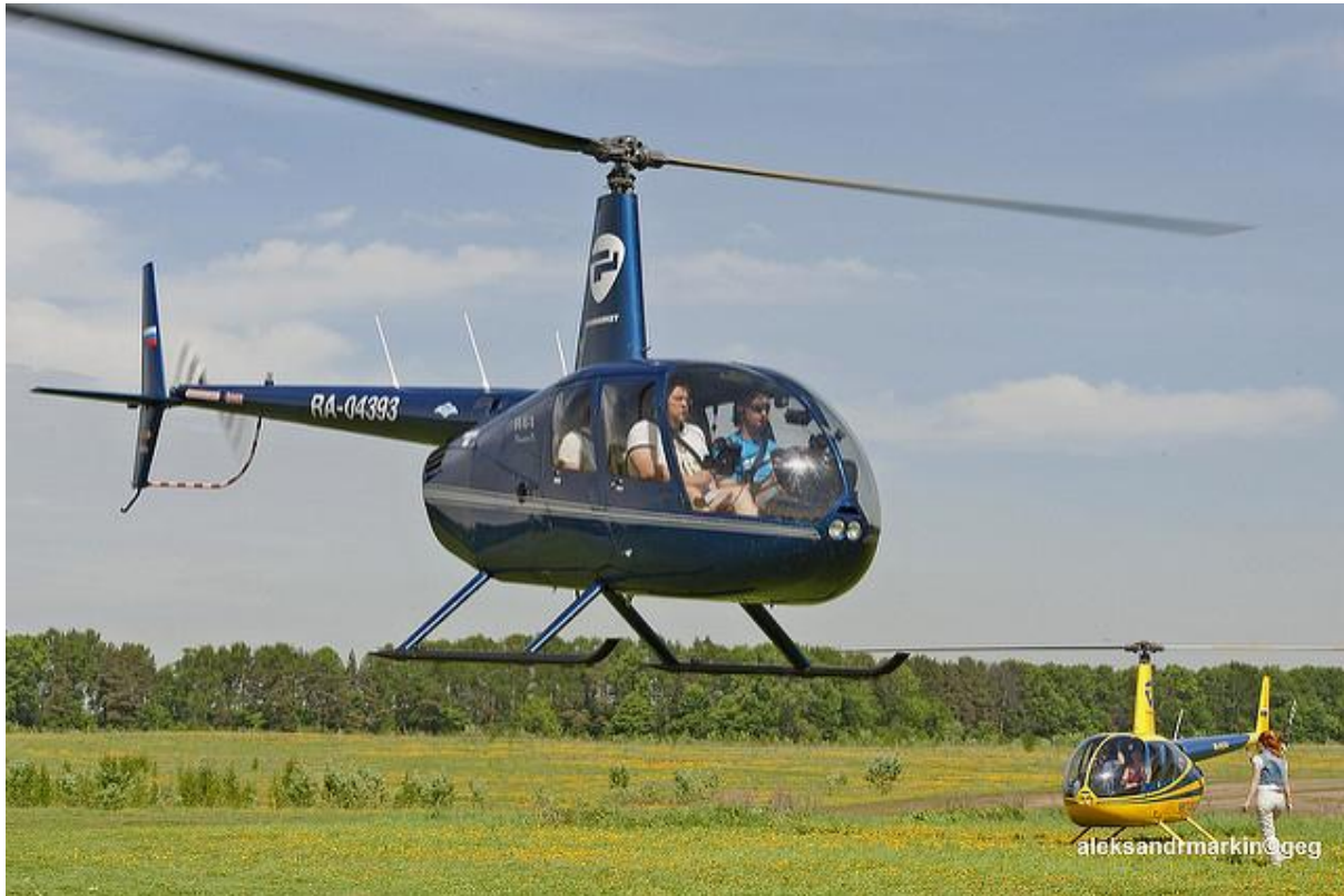
The Robinson R44 uses AvGas instead of Jet A. Image credit: Flickr user Aleksander Markin. Александр Мар. ( CC by 2.0 )
